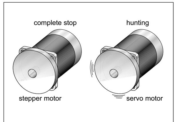
At motor stand still the stepper motor completely stands still (left picture).
