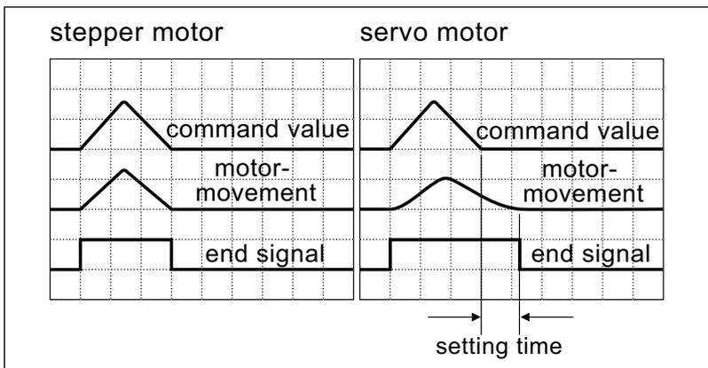
The stepper motor follows its position command values immediately (left picture).
