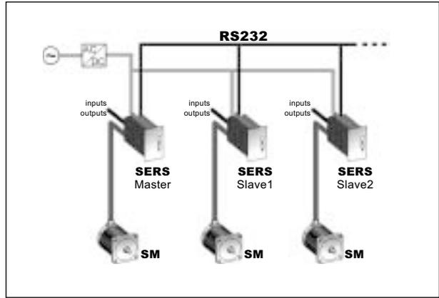
Operation with a SERS as higher order intelligent control (master), which controls other SERS-slaves via the serial interface.
