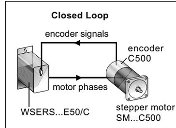
By using Closed Loop control the stepper motor can be operated always with its maximum torque.
