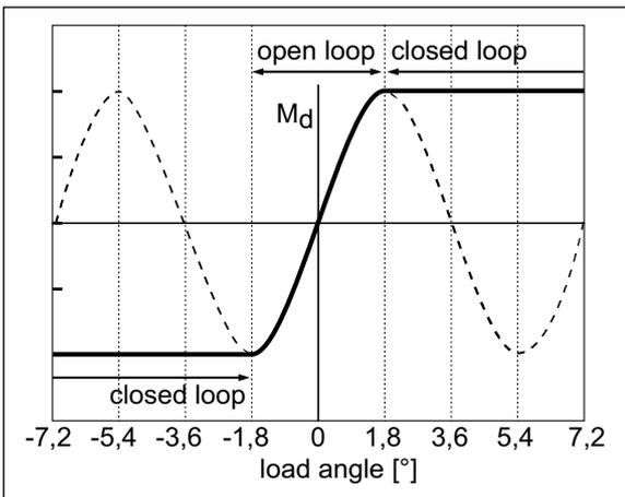
As long as the load angle is  $<1,8^\circ$ , the stepper motor will be operated in open loop mode.
