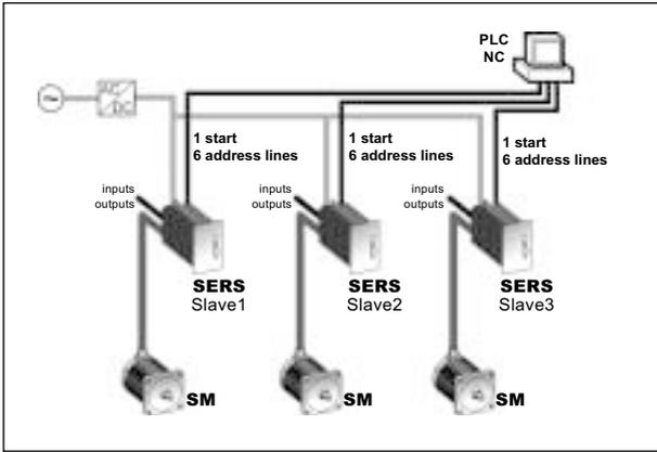
Operation with a PLC/NC or simple switches as higher order control, which call and start different operational programs in the SERS via the digital-parallel inputs (binary mode). Up to 64 different operational programs per SERS can be called.
